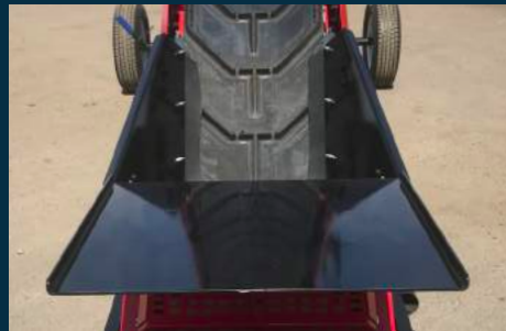
HOPPER DECK WITH BLADE
